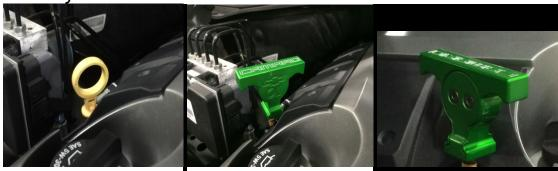
3.Orient the windshield washer cap over the existing cap and press down to snap into place.
