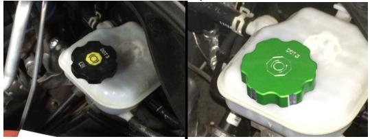
5. Remove the tape backing on the inside of the master cylinder cap. Press the cap over the existing cap and hold down for 2-3 minutes to ensure adhesion. 6. Repeat step 6 for the oil fill and radiator caps.
